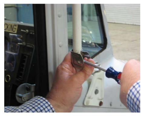
3. Turn the clamps 180° and reinstall them over the mirror support loop. Apply hand force and squeeze clamp tabs together.
