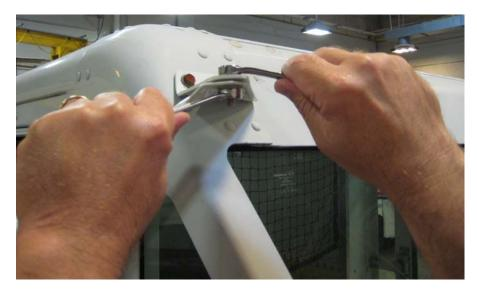
5. At the breakaway assembly, hold the top bolt head stationary and loosen the locknut 1/4 turn.
