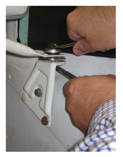
6. Rotate the mirror support loop rearward. If the lockplate remains stationary, loosen the bottom locknut an additional 1/4 turn and try again.
