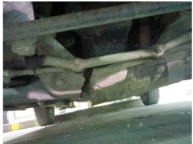
An LLV with a broken frame used to deliver mail in the Western Area
